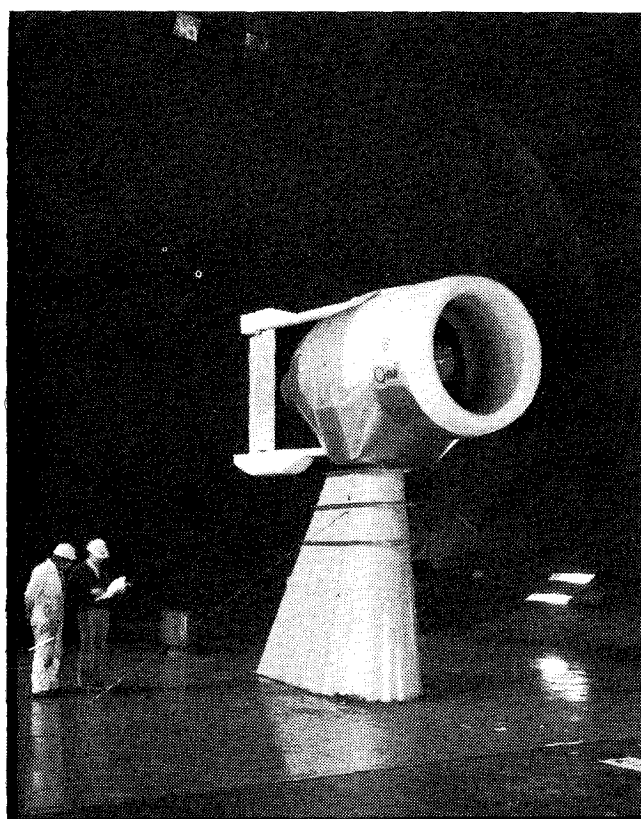
Fig. 2 Tilt-nacelle V/STOL propulsion system with control vane in the Ames 40 × 80 ft wind tunnel.
